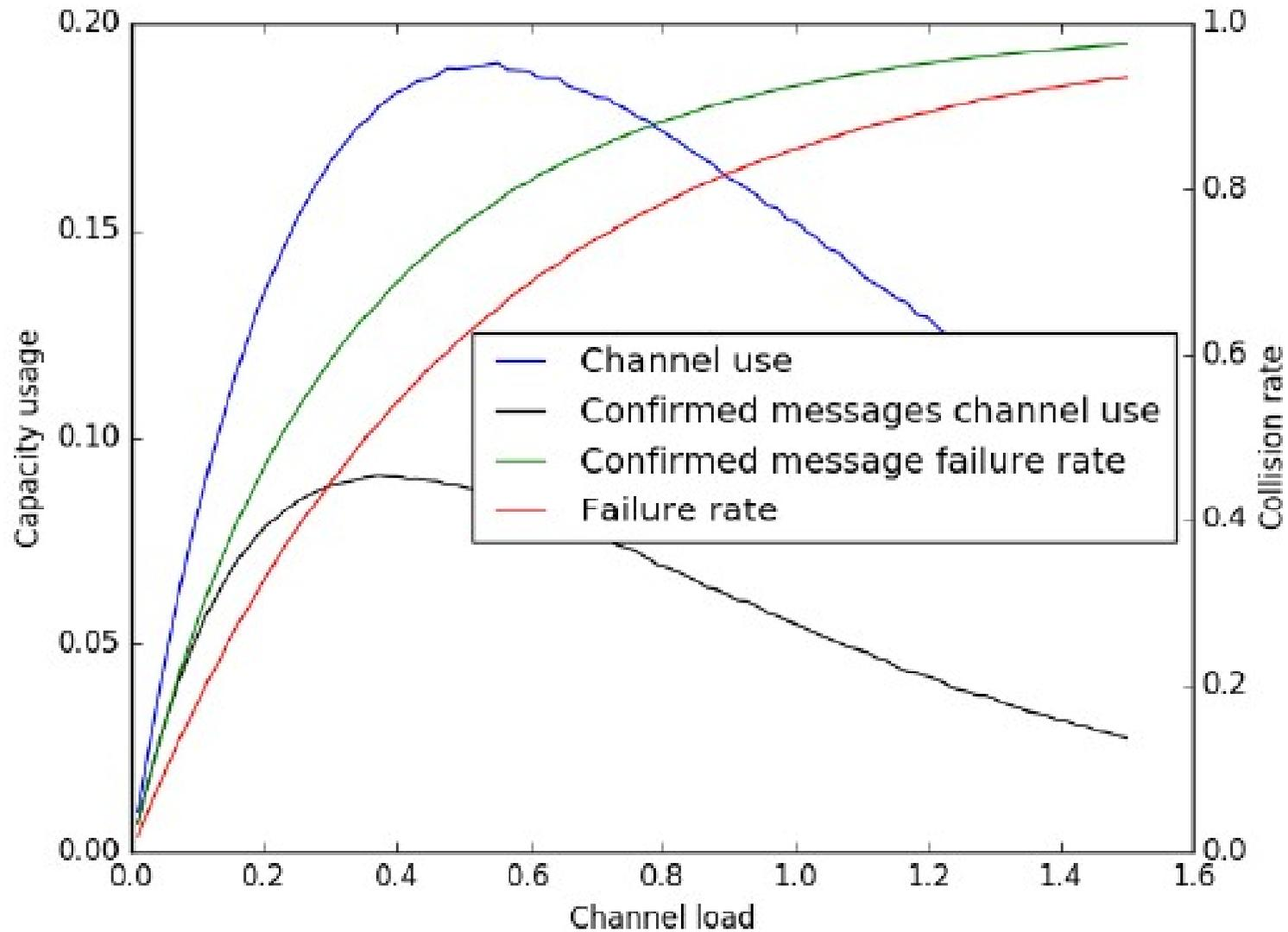
Link capacity usage and packet collision rate for a LoRaWAN network when using confirmed messages
